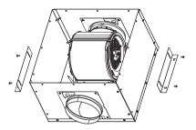
Mark the hole dots on the fixing surface. Use a ø8 mm drill. Insert the raw plugs (supplied with the kit).
