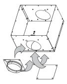
Otherwise it is necessary to prepare a hole at the rear part of the hood and place the junction box in that position considering that it has to be easily reached in case of possible service interventions. Fixing of the box has to be carried out from the outside of the hood.
